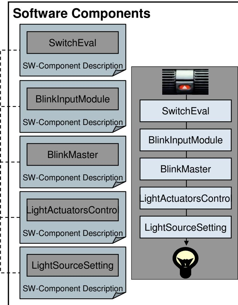
**The system configuration maps software components to ECUs and links interface connections to bus signals.**
